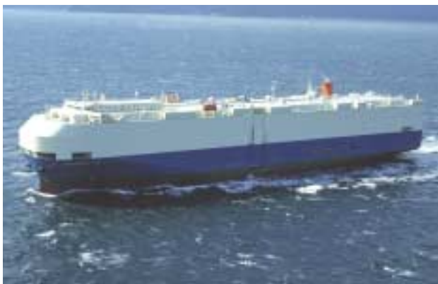
The pure car and truck carrier "Courageous Ace" designed to reduce wind resistance
