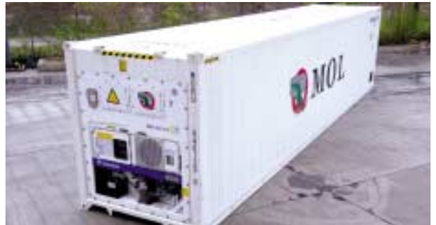
Refrigerated container using R-134a
