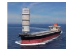
The coal carrier Shofu Maru equipped with Wind Challenger (hard sail wind propulsion system)
