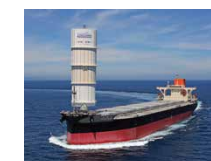
The coal carrier Shofu Maru equipped with Wind Challenger (hard sail wind propulsion system)
