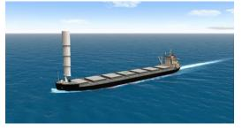
\* The Wind Challenger is a telescoping hard sail that converts wind energy to propulsive force. Installation of the system on merchant ships has the potential to significantly reduce fuel consumption, which in turn reduces the environmental impact of vessel operation while improving economic efficiency.
