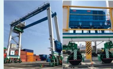
Demonstration of converting cargo-handling equipment to hydrogen fuel cells (Yokohama Port)
