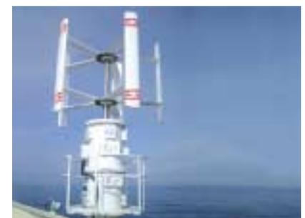
Windmill installed aboard the TAIHO MARU during practical tests of the wind power generating system Photo2
