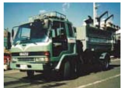
This mobile washer cleans cargo containers with water and detergent **Photo6**
