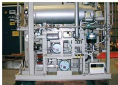
Ballast water purification experimental system
