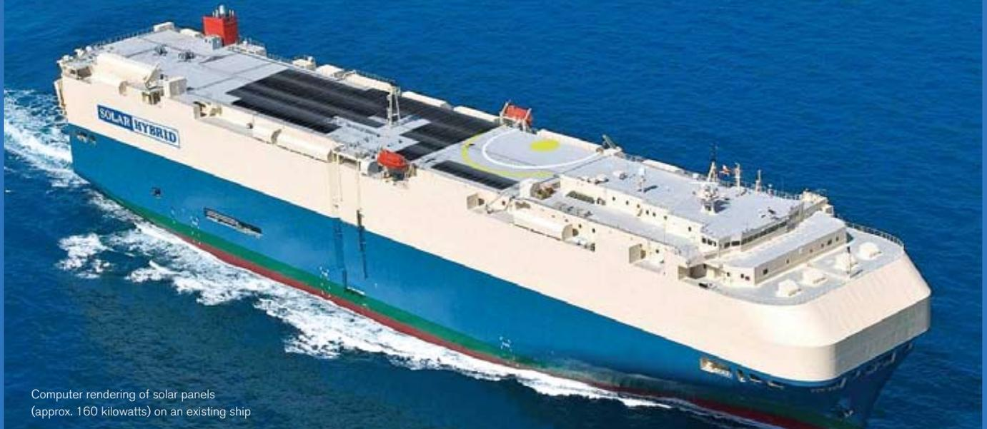
Computer rendering of solar panels (approx. 160 kilowatts) on an existing ship
