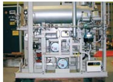
Ballast water purification experimental system
