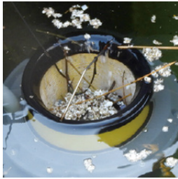
Seabin installed at Hiroshima Municipal Pier
