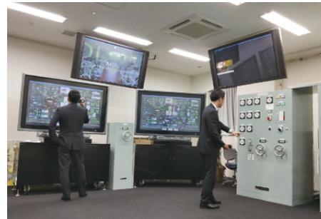
Engine Simulator equipped with actual control device
