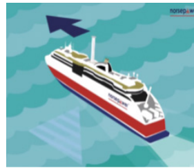
The pressure difference causes a lift (thrust) force perpendicular to the wind direction.
