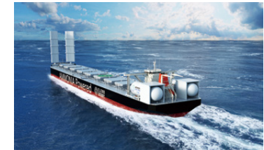
CG rendering of the 210,000 DWT ammonia-powered bulk carrier
